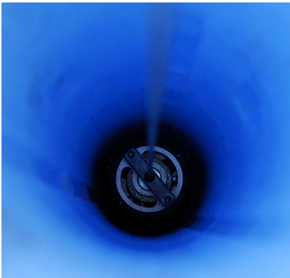
Old ice holds a memory of the ancient atmosphere. The Million Year Ice Core Dome C North borehole will eventually extend over three kilometres deep beneath the ice sheet to the Antarctic bedrock. Photo: © Joel Pedro/AAD
